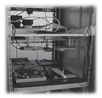
Figure 2 Mounted remote laboratories (FPGA, Microprocessor and PIC)
