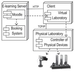
**Figure 5** Deployment diagram (UML)
