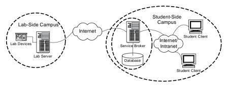
**Figure 4** Topology of the Batched Architecture [1]
