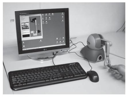
**Figure 10** MMC Hybrid system using haptics interaction [20]
