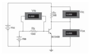
Figure 7 Schematic circuit to test the BJT
