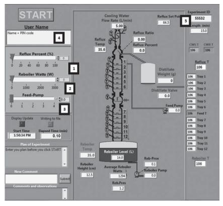
Figure 12 Control Panel of Distillation Column
