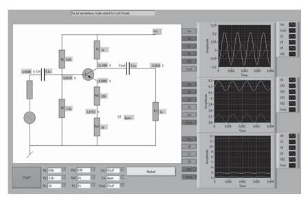
Figure 2 Screen capture from the BJT remote laboratory
