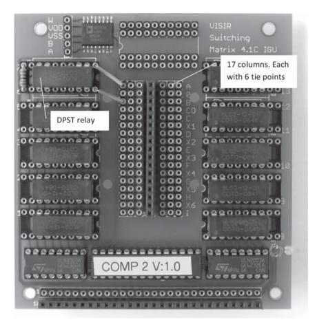
**Figure 7** A component board
