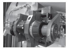
Figure 17 Self developed automated clamping unit (force and distance controlled)
