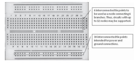
Figure 2 A solderless breadboard
